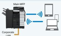
Up to 5 devices can access bizhub C368/C308/C258 simultaneously in AP mode with UK-212 equipped. Up to 4 devices can access bizhub C368/ C308/C258 simultaneously in Simple AP mode with UK-215.
